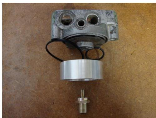
Remove the original filter bowl and its sealing ring (which may be stuck in the filter head). If fitted, remove the splash plate (this looks like a large steel washer) in the centre of the filter head. If there is a felt washer under the plate remove this also. Fit the large sealing ring supplied into the groove in the filter head.
